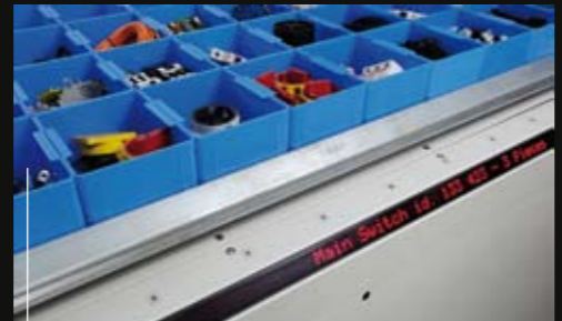
An optional position indicator displays the description, location and quantity of goods to be picked.
